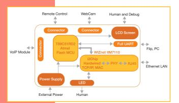
with Atmel 80C51 Flash MCU and the WIZnet i2Chip®, a unique hardwired embedded Ethernet TCP/IP chip.
